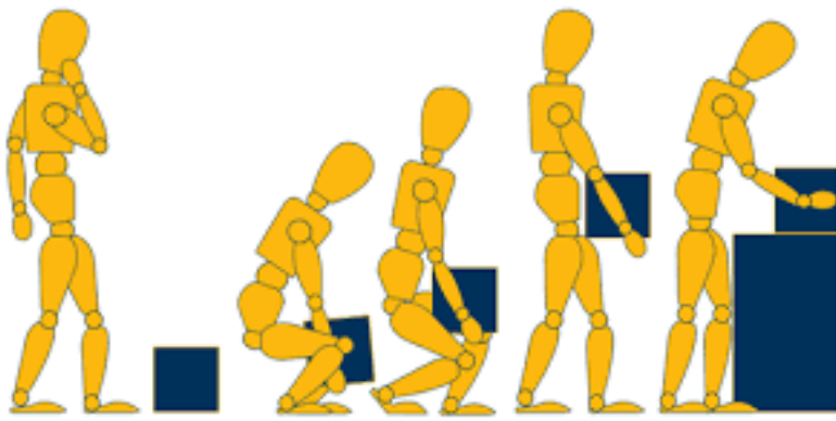
Figure 4: Illustrates the correct lifting technique
